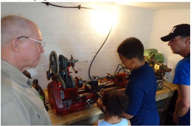
In this photo the young visitor continues the facing process for the end of the piece of plastic stock. This lathe was built about 1940 and was used in the Linden NJ General Motors Plant to manufacture landing gear parts for Navy F4F Wildcat fighter planes.
